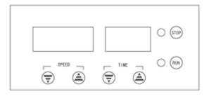
III. Take an oscillator controller as an example to illustrate the function of each key(maximum timing is 999 minutes)
