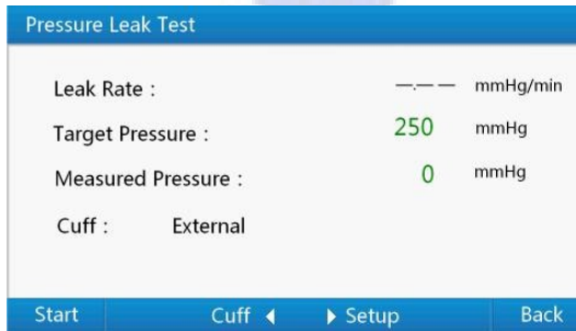
Figure 10 Pressure leak test interface
