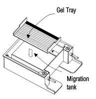
**4.3.2** Pour buffer solution to a level of about 3mm above the surface of the gel,250-300ml of buffer is required.
