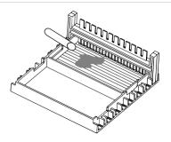
**4.2.3** Hold the two sides of comband pull out slowly after the gel solidified. The hole of gel shouldbe ordered and without damage.
