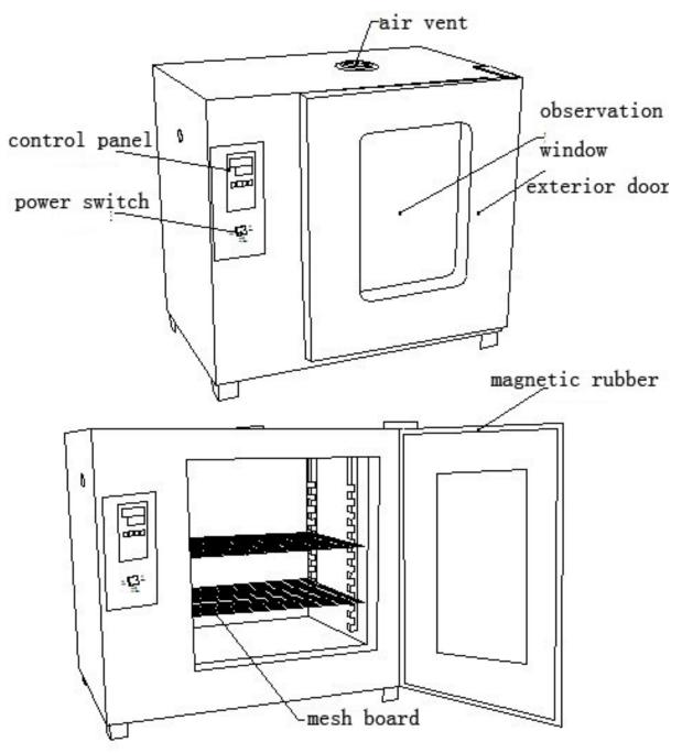
Shell is made of steel plate, and spray paint treatment. Inner chamber is made of zinc-plating or stainless steel. the observation window is double tempered glass
