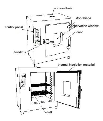
Heating wire is in the bottom of inner chamber, fan in the left of chamber. controller controls the constant and change of temperature, the air flow inflows inner chamber via heating wire, and the function of fan is to make inside temperature more uniform. arc-design, shelf space can be adjusted, built-in temp. probe. The inner chamber is made of zinc-plating or stainless steel. Observation window is tempered glass.
