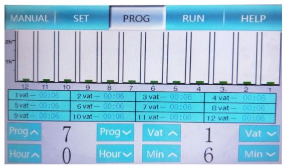
Touch program  $\blacktriangle$  and  $\blacktriangledown$  key, can select 20 sets program. After confirming, press the number of the container  $\blacktriangle$  and  $\blacktriangledown$  key, select the number. Touch hour  $\blacktriangle$  and  $\blacktriangle$  key, can set the socking time (0~24) of per container. Touch minute  $\blacktriangle$  and  $\blacktriangledown$  key, can set the socking time (0~59) of per container.
