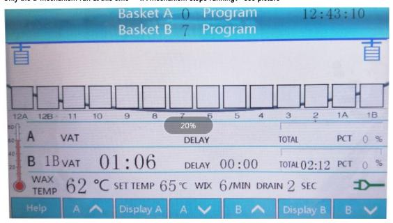
When you want to restart the A mechanism, please enter the press the set button entering the setting interface after turn the equipment. Press the A mechanism start button. The A mechanism will get to the 1A container automatically. Please see the following picture.
