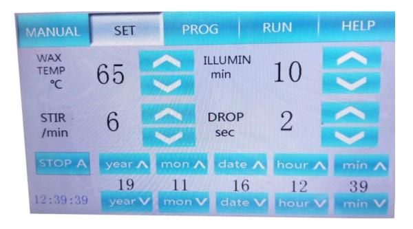
The paraffin container temperature can be set 0-80°C, the illumination time can be set 1-30 minutes, the stirring frequent can be set 0-6 times /minute, drop time can be set 10-30 seconds. Total time and completion time are
