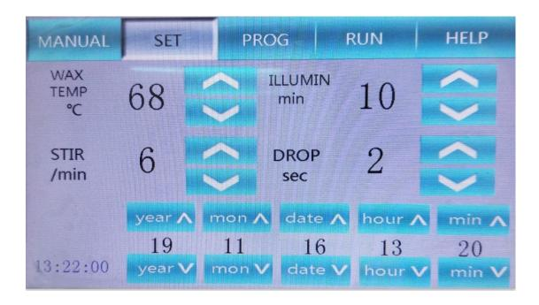
If it is power off when the program is running, the mechanism is going to the 9<sup>th</sup> container, it will go the protective container automatically.
