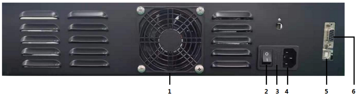
1. Cooling vent 2. Power switch 3. Fuse holder 4. Power socket 5. USB port 6. Printer port
