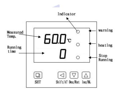
3. temperature sensor, if the upper screen displays"----", it means that there is something wrong with temperature sensor or temperature is outside of measure range or controller fails, controller will cut off heating output automatically, and with continuous beep, alarm indicator is on, please check temperature and connection.
