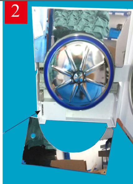
2. You will see the screws that fix the door handle.
