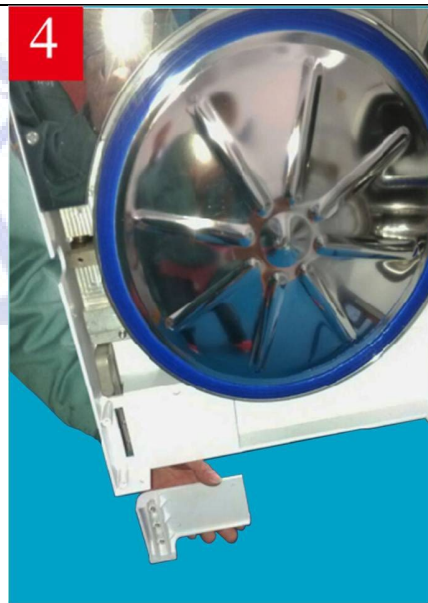
4. Take the door handle from the bottom and replace it.
