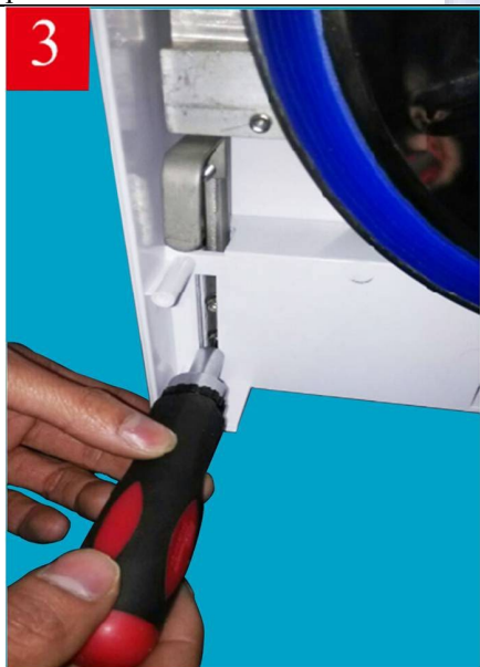
3. Remove the screws.
