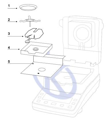
Please installation the instrument according the picture Installation order from top to bottom :1 --2--3--4--5
