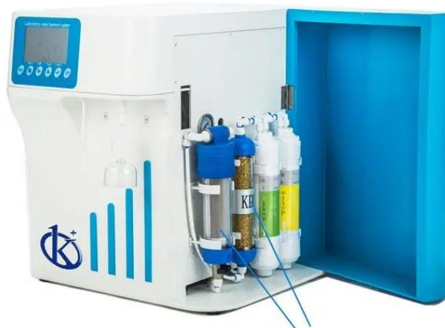
Inside part of the machine, pre-filtration elements
