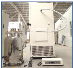
LN 2 /CO 2 backup system
